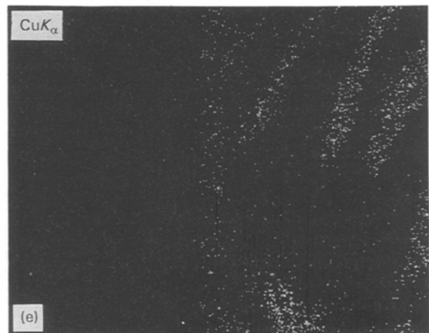
Figure 5. Images of (a) SEM and of (b–e) AlK α , AgK α , TiK α and CuK α X-rays at the same area heating at 1173 K for 1.8 ks.
